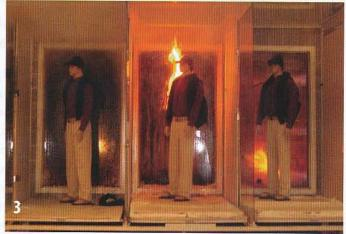
Here are photos of independent testing on 3 types of fire protective glazing to demonstrate effects radiant heat.
