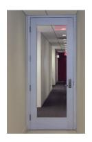
The GPX Architectural Series 20 minute fire protective aluminum door is a full vision, stile and rail door that incorporates SuperLite I clear specialty tempered glazing. SuperLite I with PPG Starphire® Ultra-Clear Glass and SuperLite pattern glass are also available glazing options. Fully listed and labeled by Intertek-Warnock Hersey, this product meets NFPA 252, UL 10C for positive pressure, and CPSC Cat. Il impact safety (with SuperLite I glazing).
