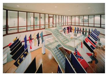
SuperLite II-XL 60 and GPX Architectural Series Framing were used to create a transparent wall system that seamlessly combines vision and light with maximum fire protection. This fire rated system also provides smooth, angular transitions along the corners to achieve the designer's intent to have a beautiful viewing area that highlights the building's focal point.
