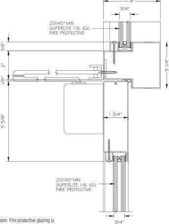
\* AHJ approval required for 45 minute applications because it is tested without hose stream. Fire protective glazing is limited to 100 sq. in. in temperature rise doors and up to max. size tested in non-temperature rise doors. Fire protective glazing is limited to 25% of the wall area and cannot be used in applications that require ASTM E119 or NFPA 251.
