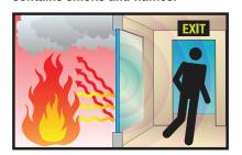
Reflects radiant heat back to the fire source, allowing safe egress in corridors.
